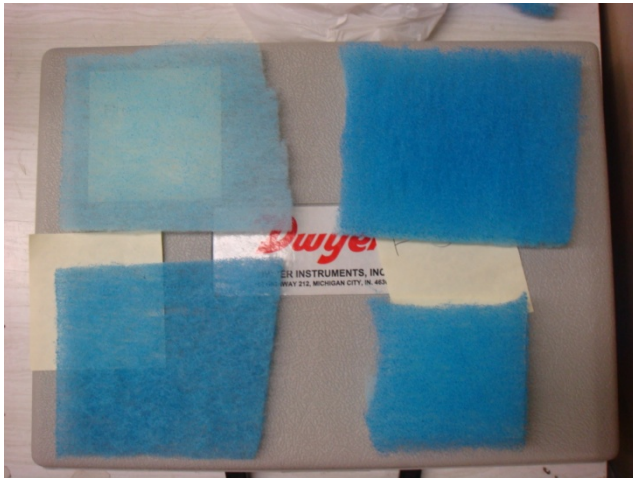
Figure 6 | Clockwise from left upper corner: fiber filter 1, 2, 3, and 4. Filters 1, 2, 3 are of same size. Filters 1 and 2 are about 1 cm thick. Filters 3 and 4 are of same thickness, about 2 cm thick
